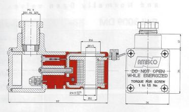
**The product** is developed to be used in ambients with temperature range from -50°C to +50°C, and it has a power consumption of 3.8W for type T4 and 3W for type T5.
